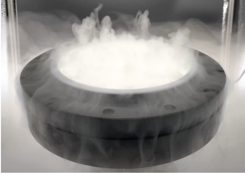
Flow Test of the Catalytic Honeycomb in the Burner Prototype
