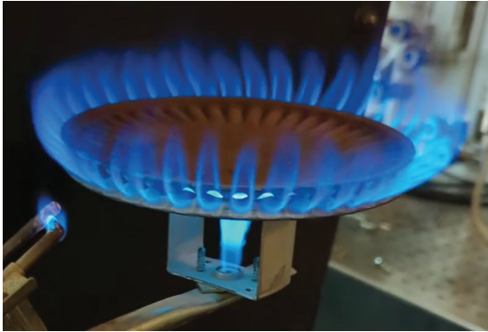
Flashback in conventional burner
